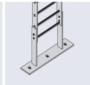
Spreader Plate Feet base fixing
